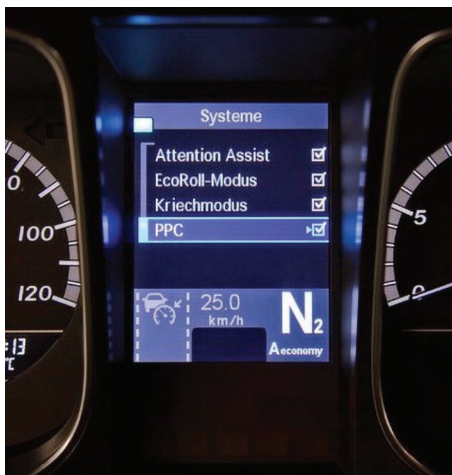
Predictive Powertrain Control (PPC) allows additional fuel savings. Combines digital 3D maps, GPS information & high performance computer.
